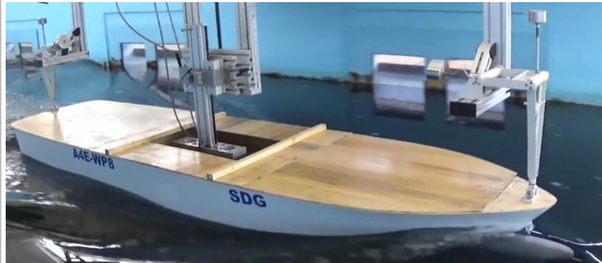
Figure 1: Experimental model during towing tank tests
